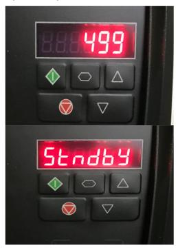
When the drive is linked to the mains power, the drive will test the pump by setting this to 499 RPM and then back to 0.
