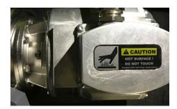
Be careful: the surface of the pump can be very hot (up to 75 °C). Do not touch it directly before checking the surface temperature. For the pump itself, this temperature is normal and no problem. Always ensure good ventilation around the pump.
